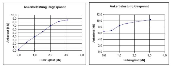
Fig 3 Experimental results of measurements of anchor point force
