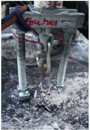
Fig 14 Axial pull of an anchor with the tensile tester
