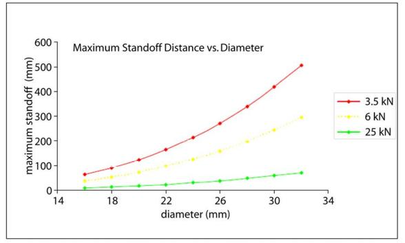
Fig 13 Graph of stand-off distance vs. anchor diameter
