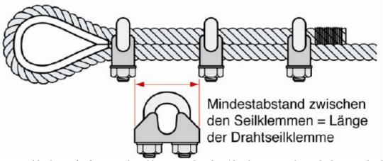
**Fig 20** Cable clamps for fastening the cable to an end anchor (the clamps must be applied to an unloaded section of cable). "The minimum separation between clamps = the clamp width" **Fig 21** Eye grommet/stiffener in a cable loop (the first clamp must be located directly behind the grommet to prevent it from ripping out)
