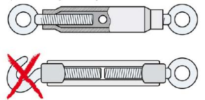
**Fig 22** Turnbuckles for wire cable (above, tube turnbuckle with eye mounting; below open turnbuckle with hook (left) and eye mounting—not recommended)
