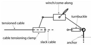
Fig 23 Sketch of how to tension cable
