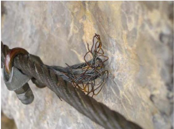
Fig 27 Defective cable
