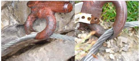
Fig 18 Friction wear of eyebolts.
