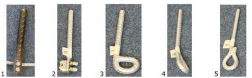
1 32 mm U-clamp anchor 2 20 mm U-clamp anchor 3 20 mm eyebolt (mfr. Schiestl) 4 16 mm angled eyebolt 5 16 mm eyebolt Fig 7 Types of anchors:
