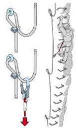
**Fig 4** The French system with cable loops in eyebolts
