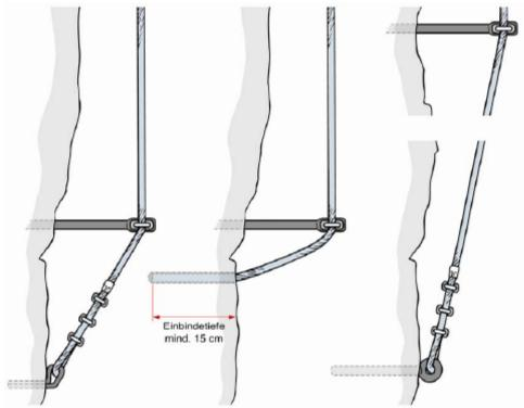
**Fig 10** End anchoring with minimal lever arm (left & right); the direct fixing of the cable to the cliff shown in the middle figure is indeed sufficient though obviously the cable cannot easily by swapped out.
