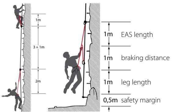
**Fig 15** Schematic diagram of a fall on a VF/KS. The separation of anchors should not exceed 4 m, and groundfall should be prevented.
