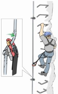
**Fig 8** Classical/east-alps VF/KS system with eyebolts and pretensioned cable (the VF/KS carabiner is loaded perpendicular to the spine axis)
